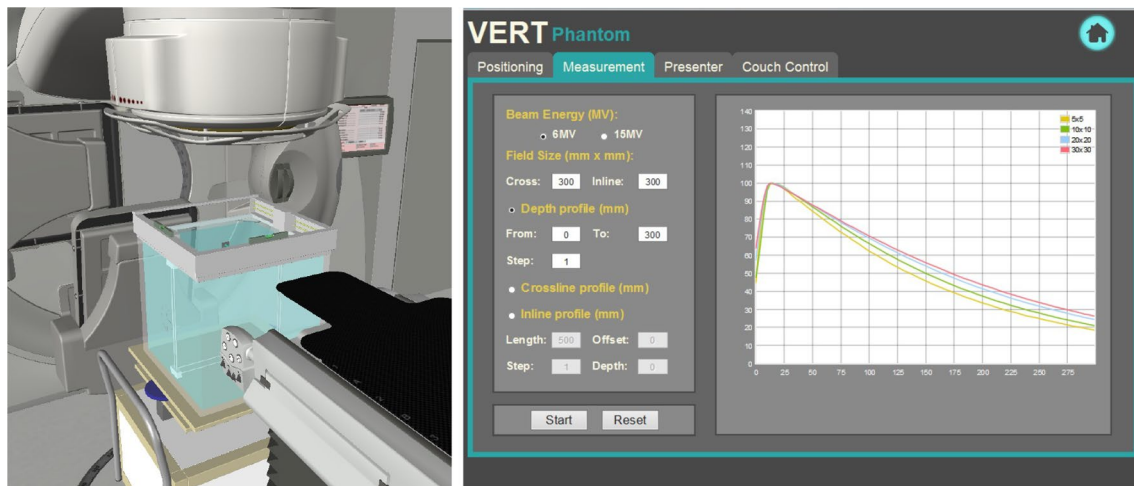
Fig. 3 Screenshots from the “Linear accelerator measurements” VERT tutorial showing water tank (left) and dose measurement profile (right)
